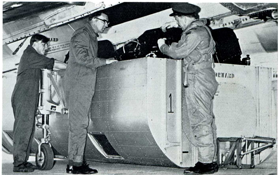
Below: The complete crated assembly of photographic equipment is ready to be hoisted into the bomb bay. On the left are photographers SAC A. Foden and Corporal W. R. Burgoyne.
